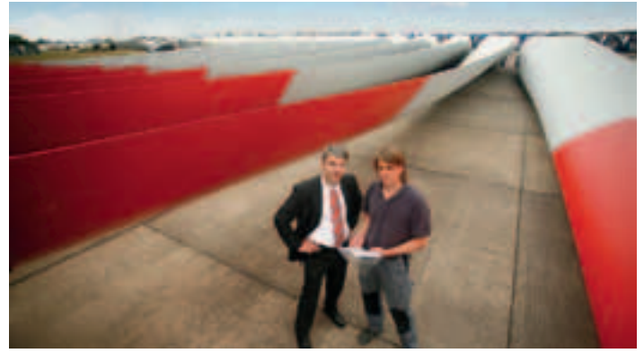
Good tailwind for composites: SGL Rotec uses CFRP for wind turbine rotor blades
